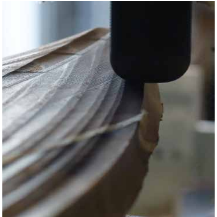
CNC machine cuts a blank into the outline of a surfboard.
