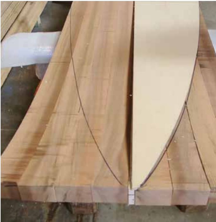
Wooden strips are glued together to make a surfboard blank.
