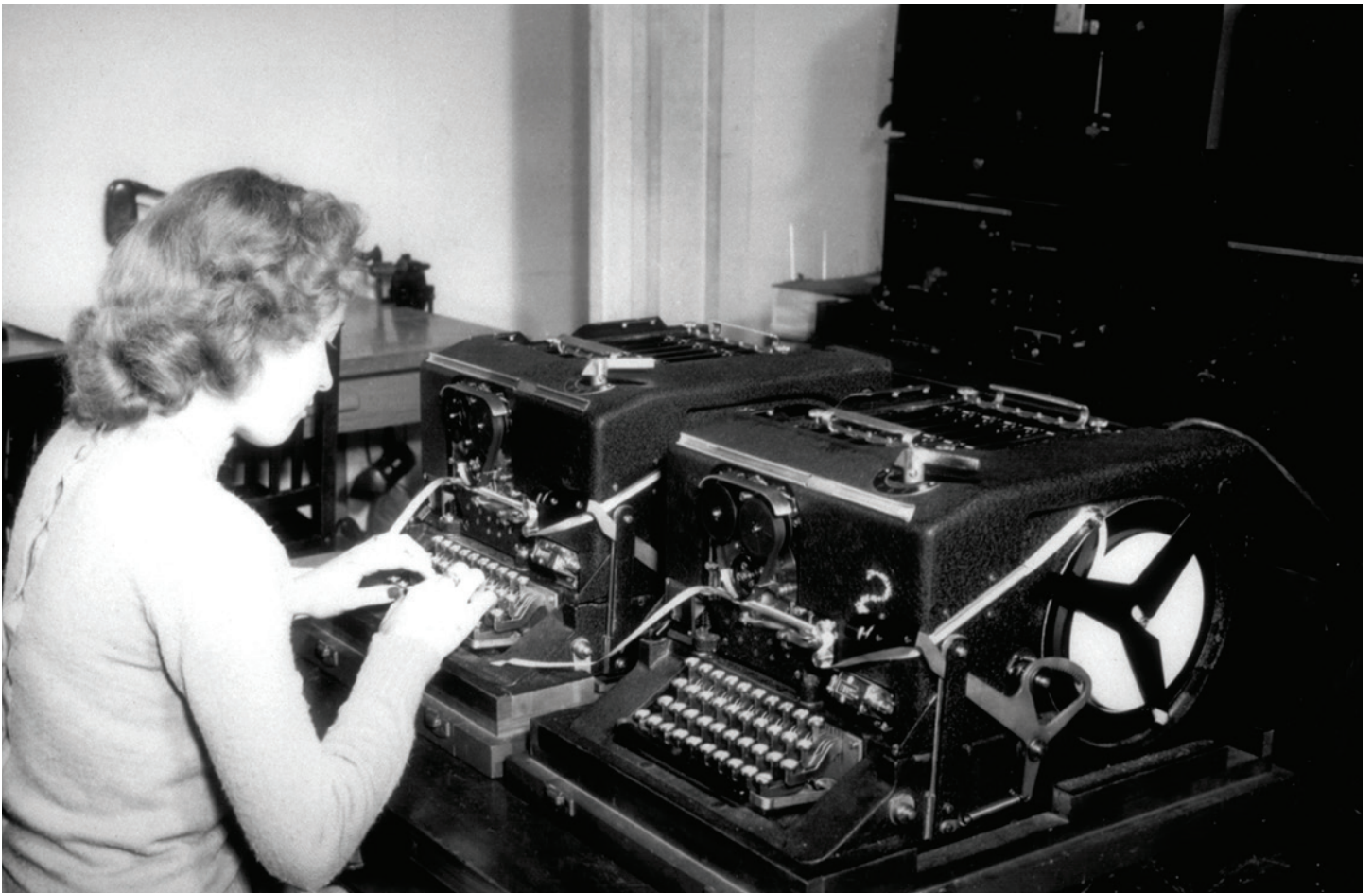
A woman operates a foolproof American SIGABA cipher machine, decrypting messages, and intercepting and forwarding enemy coded messages c. 1944
